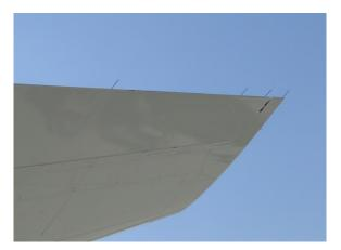
**Figure 5.** Two static dischargers missing from starboard horizontal stabilizer
