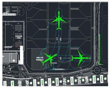
**Figure 11.** Approved pushback sequence off Stand G17 into the hatched area directly behind Stand G17, and then pull forward to the engine start line
