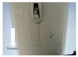
Figure 2. Damage to aft fuselage
