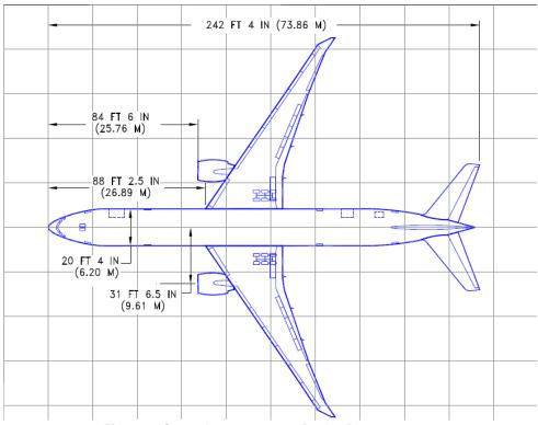
Figure 8. General arrangement – Boeing B777-300
