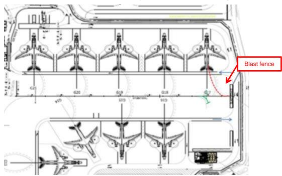
**Figure 1.** Configuration of the Golf Stands showing red, nose gear stop green, and the location of the jetblast fence
