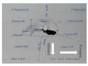
Figure 3. Detail and location of fuselage damage
