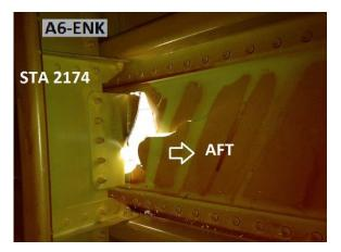
Figure 4. Internal view of fuselage damage
