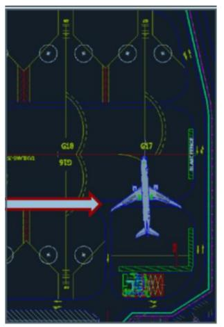
**Figure 9**. Correct orientation of the aircraft at the end of the push off Stand G17. The fuselage aft of the wings overhangs the hatched area opposite Stand G17
